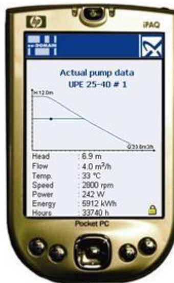
Figure 9: Pump control screen
