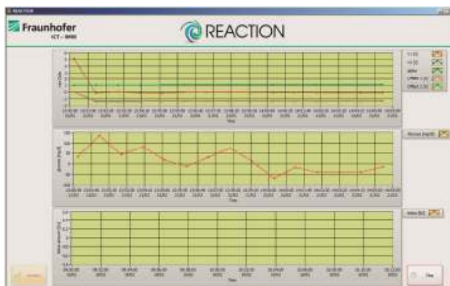
Figure 36: Graphical user interface of the IMM AGC control software, displaying the raw data of the IMM IR CGM sensor (top), the glucose concentration in mg/dl as calculated from the raw data (middle) and the bolus shots delivered to the pump (bottom), each as a function of time
