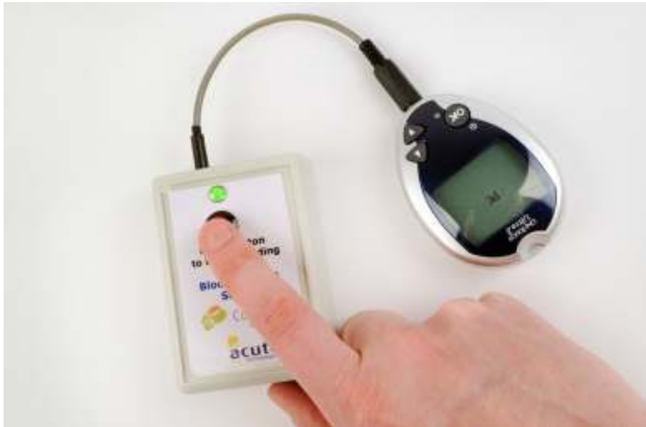
Figure 5: Blood glucose monitor extended for wireless communication
