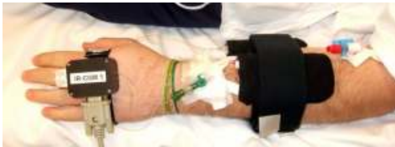
Figure 24: IMM IR CGM sensor prototype, together with microdialysis pumps, on the forearm of a patient, as applied during the clinical trials at MUG
