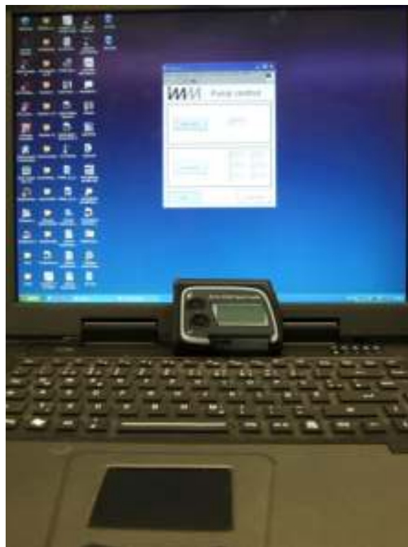
Figure 32: IMM test setup for automatic insulin pump control via PC and Bluetooth communication
