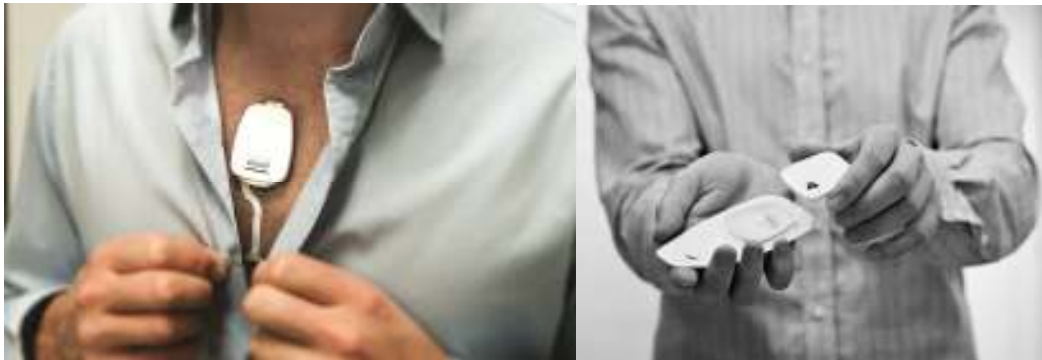
Figure 11: ePatch for ECG recording is applied on the sternum of a patient (photo on left). The ePatch monitoring system consists of a re-usable sensor that is placed into a connector on the ePatch electrode which is designed for single used (photo on right)
