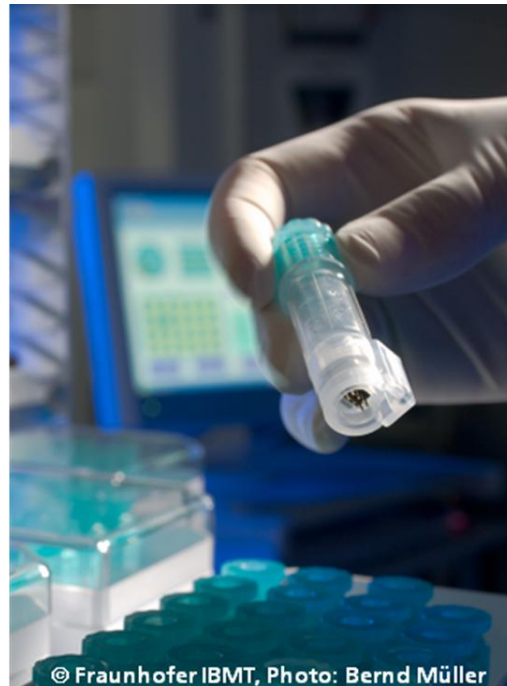
Figure 29: Smart cryo vial with integrated memory chip and RFID tag fully operational under -196^{\circ}\text{C} .
