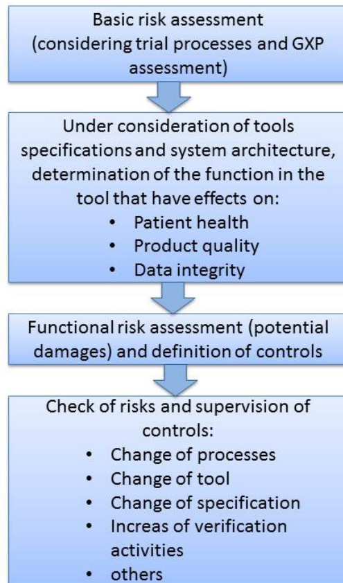
Fig 7: Hierarchy of risk assessments according to GAMP: basic risk assessment during software design phase, GCP focused risk assessment, functional risk assessment and during operations of the tool the check of risk and supervision of controls
