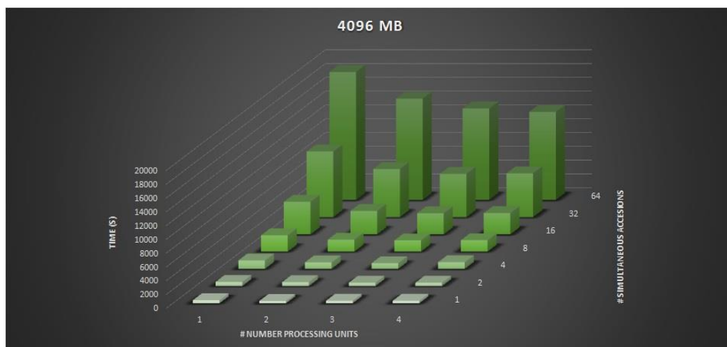
Fig A9: the response times obtained for the test# 2, with 4096MB or RAM.
