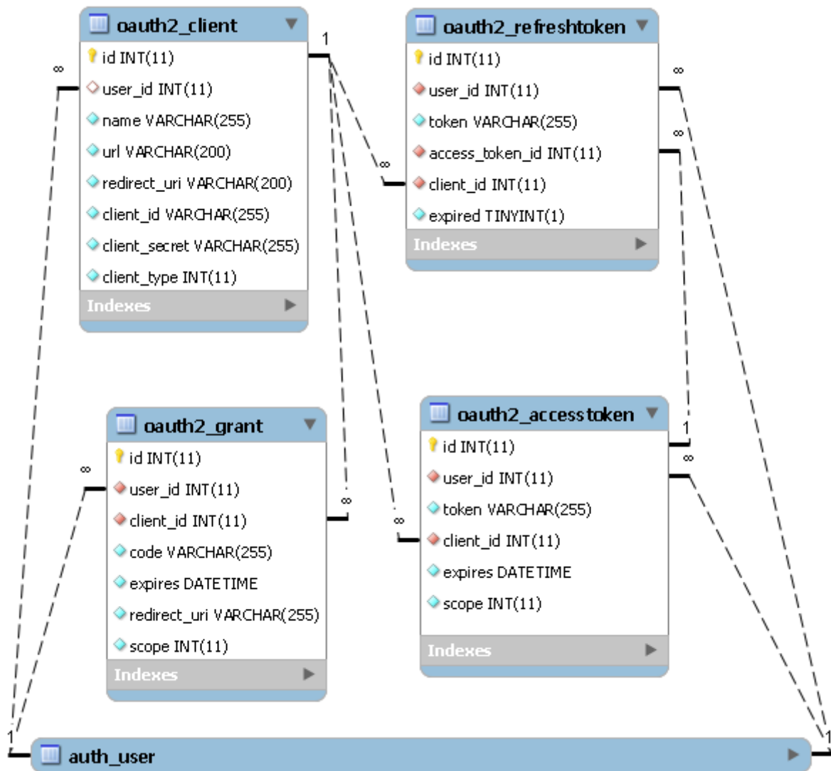
Figure 7: ER diagram of tables associated with OAuth 2.0 service provider.
