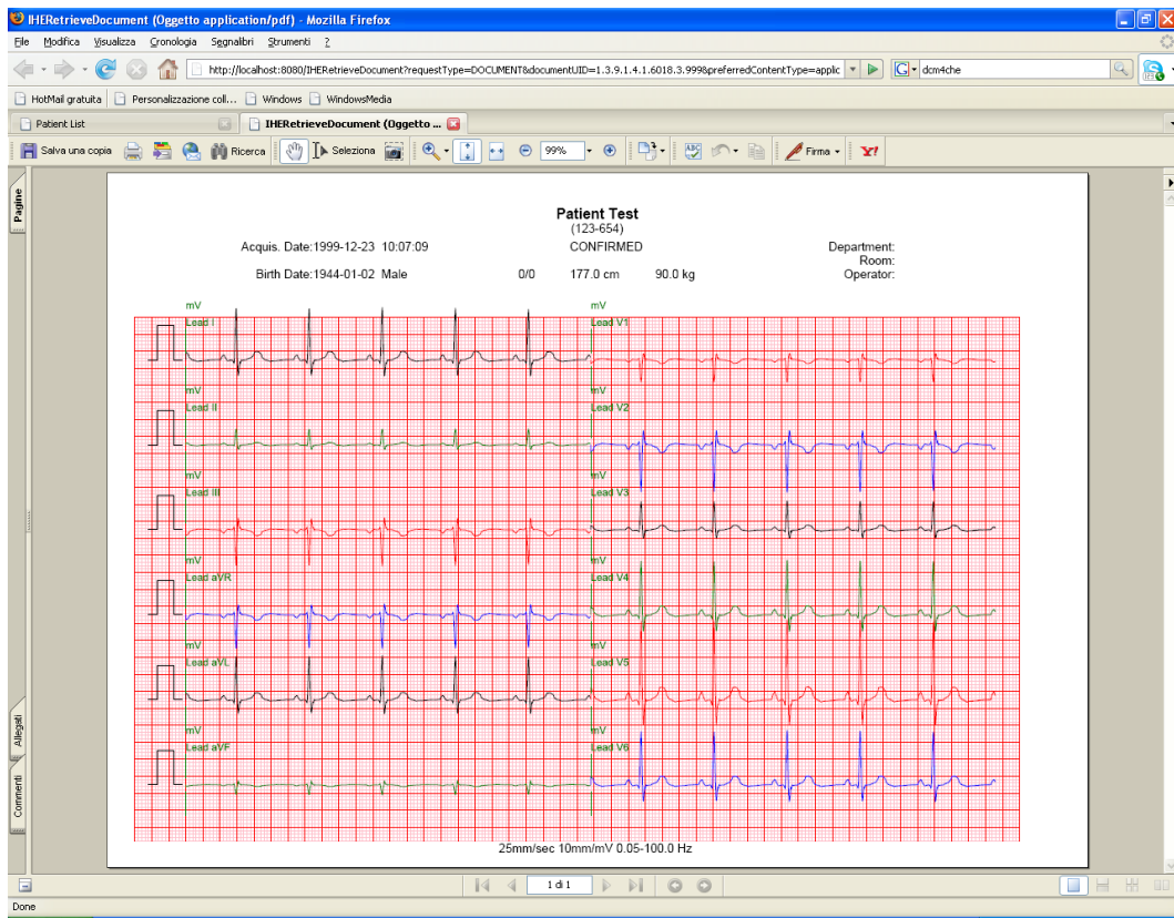
Figure 59. IHE RID of an ECG. The ECG profile is rendered as a vector graphic object and encapsulated in a PDF.
