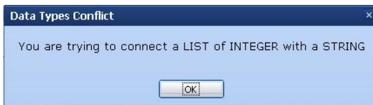
Figure 3-7 Syntactic validation of services connections
