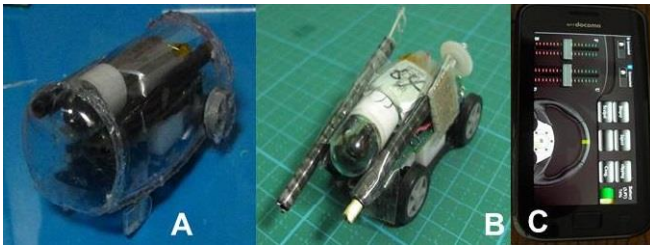
Fig.2 Two prototypes of iRoboCap (therapeutic version). A. screw-driven submarine type, B. wheel-driven amphibious type, C. Smartphone for steering.
