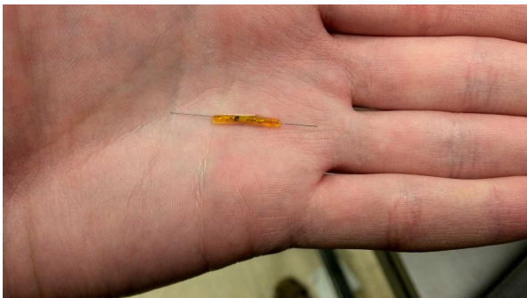
Fig. 1. (Top) Illustration of the construction of the implant. (Bottom) A photograph of the implant with platinum electrodes.
