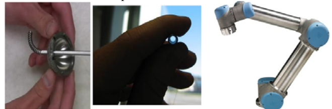
Figure 2. Snake-like Dexterous Manipulator (Left), UR5 robot [10] (Right).
