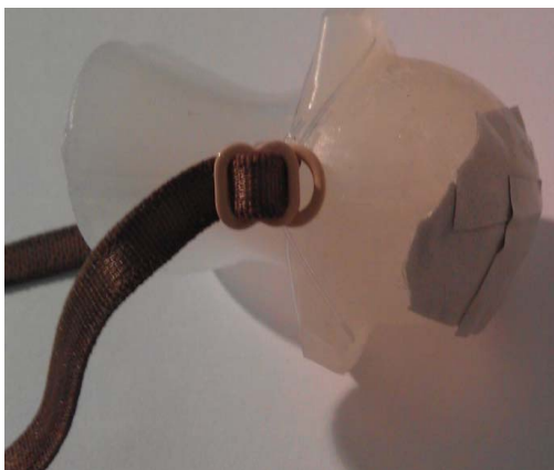
Fig. 3. Silicone tongue device with attached reflective tape
