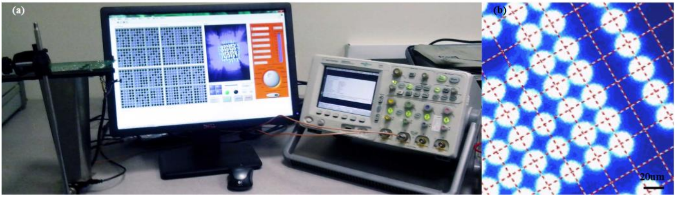
Fig. 8. (a) Stimulator prototype. The LED array is controlled by a PC interface through a micro controller. There is a high precision imager recording the stimulation patterns. The measurement results are display on the same PC in real time. (b) snapshot of measured stimulation pixels.
