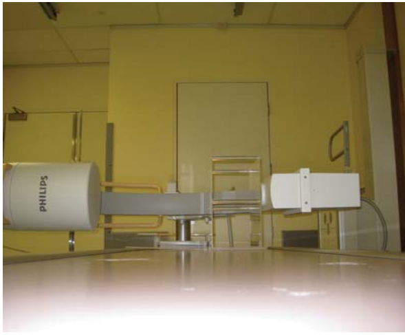
Fig. 2. 400 mm×400 mm perspex calibration box.
