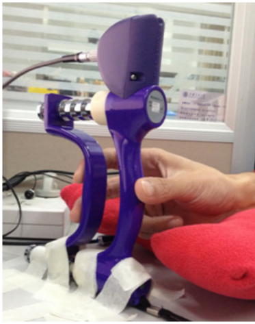
Fig. 1. Experimental Setup. The dynamometer is fixed on the table, and the cushion is placed under the wrist of the subject to make the subject comfortable. The digits are asked to put on the convex and concave part to constrain the movement.
