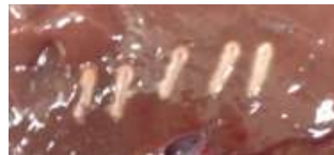
Figure 2: Bovine liver tissue ablation using prototype catheter for 3 seconds at coagulation power level 3 (~3 W). The tissue is white and shrunken in comparison to the surrounding tissue, indicative of thermal insult on collagenous structures.
