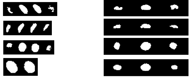
Fig. 4. Left: Selected training shapes: stacks of binary shape models of segmented nuclei selected interactively. These training shapes vary in the shapes, orientation, size and number of slices. Right: Alignment results of the training shapes. We standardized the number of image slices to three. Each training shape is scaled and translated in the z -direction such that the binary shape from the first and last slices are approximately half of the size of the middle slice.
