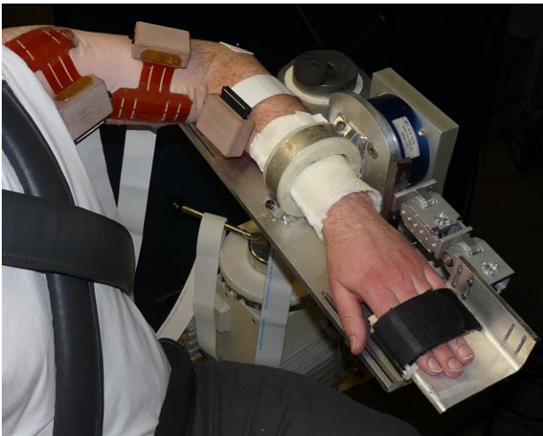
Fig. 1. Isometric joint torque recording device with high-density surface EMG grids on the deltoid, biceps, and wrist/finger flexor muscles.
