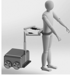
Fig. 1. The presented system is a concept design of the robot with linear actuation of \theta_2 and \theta_5 . It also shows how the patients will be connected to the chain and supported by it and the mobile base of the system components, like the tracking device for the relative feet position.
