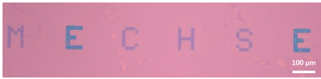
Figure 2. Optical microscope image of graphene with different number of layers. Consonant letters are composed of thinner graphite and vowel letters are composed of thicker graphite. Background is composed of bi- to tri-layer graphene on a 285 nm thick SiO 2 /Si substrate.
