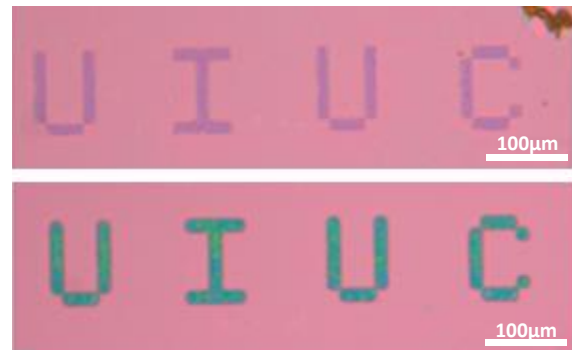
Figure 1. Synthetic control of graphene layers. Optical microscope images of graphene with different number of layers. Letters on top are composed of thinner graphite and letters on bottom are composed of thicker graphite. Background is composed of bi- to tri-layer graphene on a 285 nm thick \text{SiO}_2/\text{Si} substrate.
