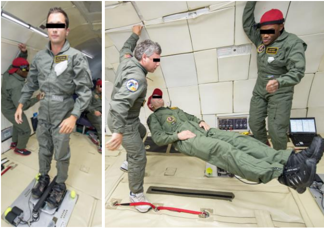
Fig. 2. Experiment setup for scale-based (left) and free-floating measurements (right). The scale was secured to the aircraft by a compressing crossbar mounted to a vibration-isolated metal plate on the aircraft frame. Free-floating subjects were manually restrained by team members.
