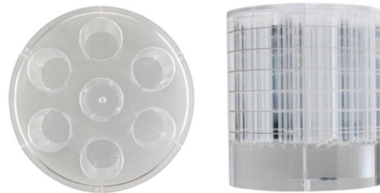
Figure 2. Image of phantom, Sendentext IQ dental CBCT. It has materials, aluminum, PTFE, delrin, LDPE for measuring contrast resolution.
