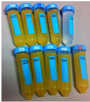
Figure 1. Picture of the phantom. Iron concentration (in \mu\text{mol/g} ) is identified for each vial (on the cap).
