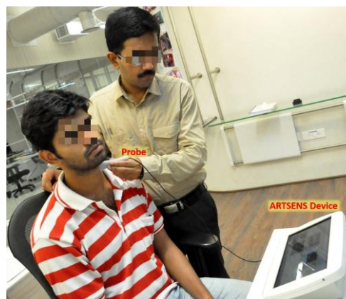
Figure 2. Measurement of carotid artery stiffness using ARTSENS
