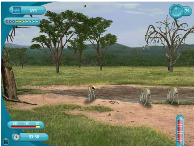
Fig. 3: Smartphone application user interface. On the right side of the screen, a respiratory guide allows users to breath at a 6 cpm respiratory rate. Cardiac frequency as well as cardiac coherence scores are visible on the top of the screen. A timer allows user to visualize the elapsed time till the beginning of the exercise.
