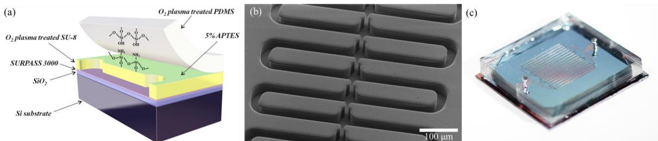
Figure 2. (a) Illustration of the microfluidic channel, (b) SEM image of the patterned SU-8 channel, (c) optical image of the fabricated device
