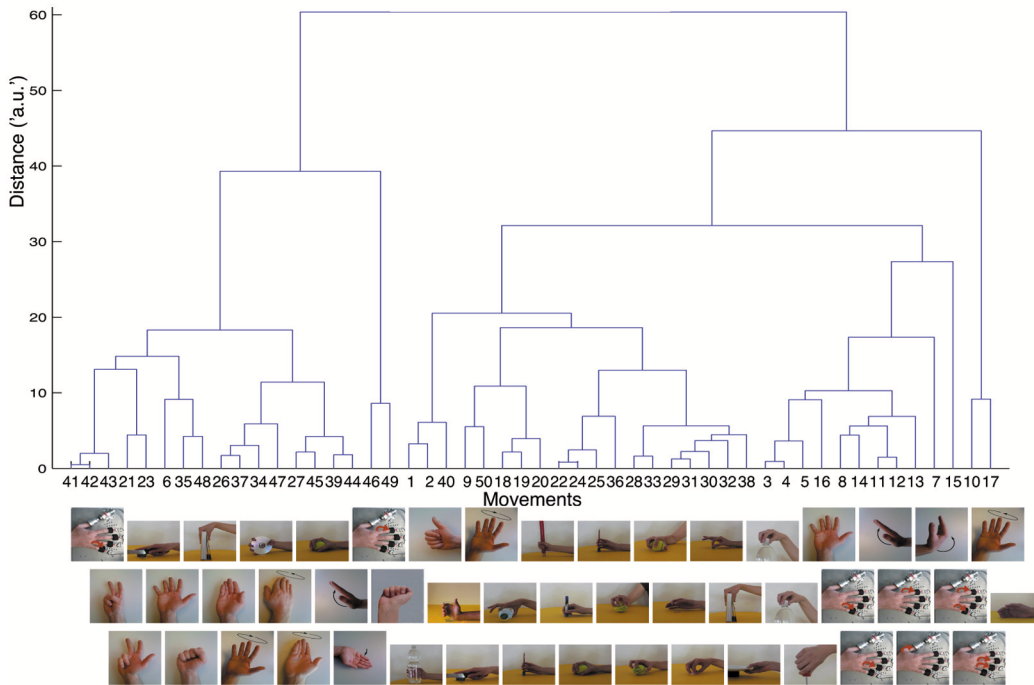
Fig. 2. Example of movement clustering dendrogram used to perform the selection of highly independent movements. Each movement number tick corresponds to the beginning of its picture below it.
