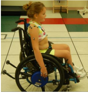
Figure 1. Subject preparing to begin motion analysis with the SmartWheel placed on subject's dominant side.
