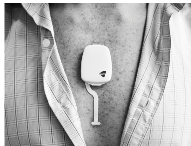
Fig. 1. The ePatch ® ECG device as worn on the sternum.
