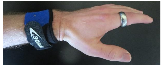
Figure 2. The manumeter is an activity monitoring device worn on the wrist that is equipped with an accelerometer for quantifying arm movement and a pair of magnetometers that quantify movement of the wrist and fingers by sensing the magnetic field changes due to a magnetic ring worn on the finger.
