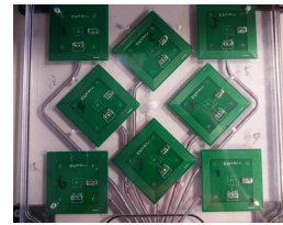
Fig. 2. The magnetic field emitter board. Eight PCB emitter coils are encapsulated in Perspex housing. The current in each coil is controlled using a constant AC current driver circuit.
