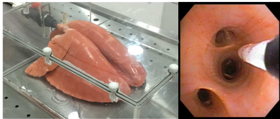
Fig. 4. (a) Plasticised pig lung when fully inflated. (b) View from the bronchoscope inside the phantom with the sensor extended out from the instrument port.
