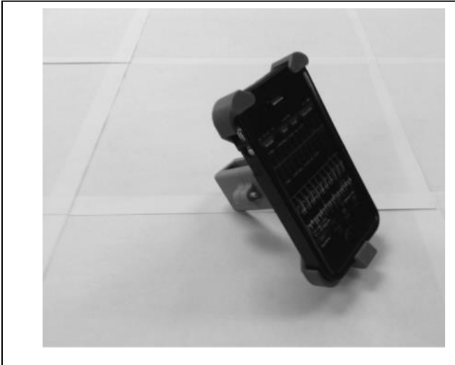
Figure 1. Smartphone (iPhone) mounted to 3D printed adapter.
