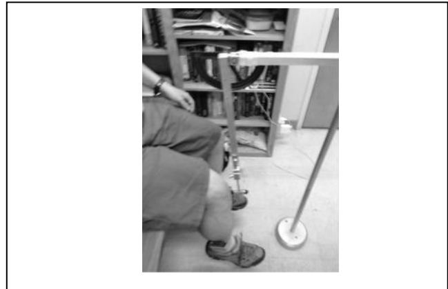
Figure 1. The experimental apparatus for quantifying the patellar tendon reflex response through a wireless gyroscope application from a smartphone. The smartphone was mounted proximal to the lateral malleolus. The potential energy impact pendulum features an attached reflex hammer.
