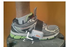
Fig. 1. Shimmer location, with coordinate system shown
