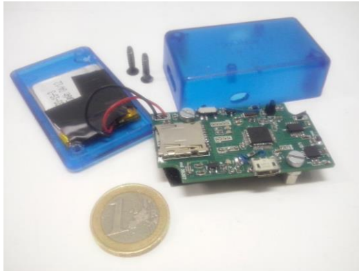
Figure 1. The assembled device and casing: battery (left) and circuit board (right).
