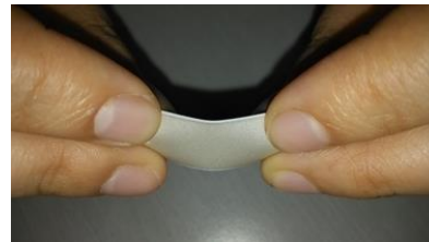
Figure 3. The piezoelectret-based sensor unit used in this work.
