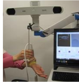
Figure1. The probe instrumented with a rigid body and camera origin system
