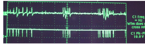
Fig. 2. Oscilloscope snapshot as verifying the spike detection circuit. The top is a raw input signal. The bottom presents the detected pulse output.
