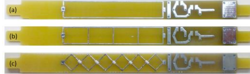
Figure 2. To validate the induced current being cancelled on the return paths of the DPPX coil, we built three trace-only coils without any capacitors. (a) Dual plane pair. (b) Dual plane pair with shorted return paths. (c) Dual plane pair with criss-cross return paths.
