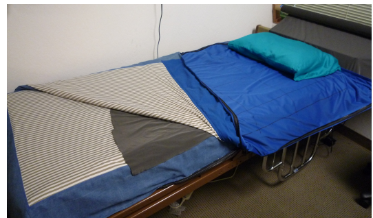
Fig. 1. The pressure sensitive bedsheet setup with sensing eTextile layers.
