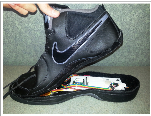
Fig. 4. Completed and functional piezoelectric energy-harvesting shoe prototype (same size and height as unaltered shoe).
