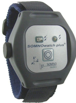
Figure 1. The Somnowatch plus that was worn by study participants. The light sensor (upper left) and the button that can be used to place a marker in the recorded data (center) are also visible.
