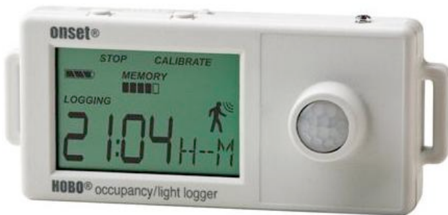
Figure 2. The HOBOWare UX90-005M Room Occupancy/Light Logger that was used during the study.
