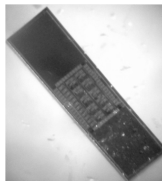
Fig. 2. Electrochemical Dual Dual mode, shared opamp Circuits fabricated in CMOS 0.18 \mu\text{m}
