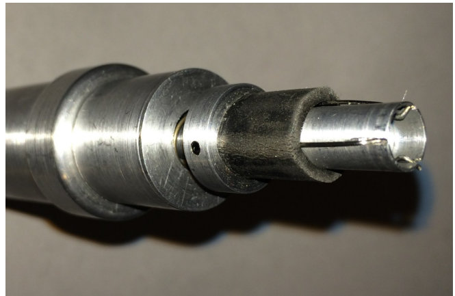
Fig. 3. Tip of Phase II device - array collet held in place by three spring clips.
