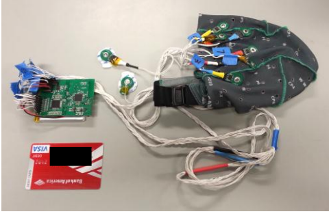
Figure 1. The EEG signal acquisition system
