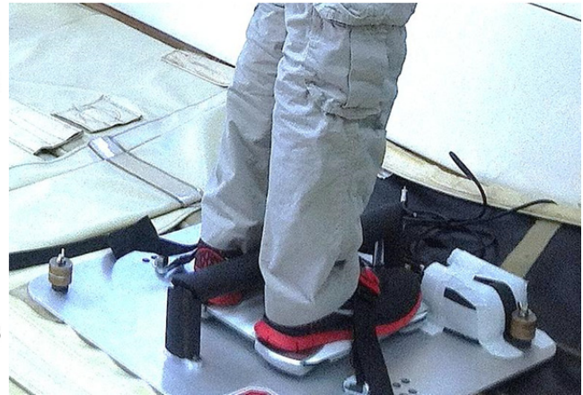
Fig. 1. Left, microgravity BCG scale setup comprised of baseplate, scale, cross beam/stanchion, and foot straps, secured to aircraft floor with four vibration isolators. Right, subject on experimental BCG setup in microgravity aircraft.
