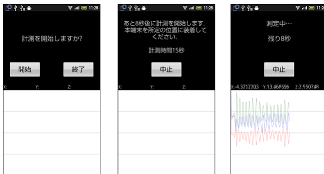
Figure 3. Gait measurement screens Left: start screen (left button is start, right is exit), Center: count down screen (measurement starts 8 seconds after, Right: measurement screen (measurement ends 8 seconds after).
