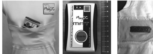
Figure 1 - The MagIC-SCG system. Left panel: the vest and the pocket containing the electronic board; mid panel: the electronic board; right panel: particular of the textile electrodes for ECG recording.
