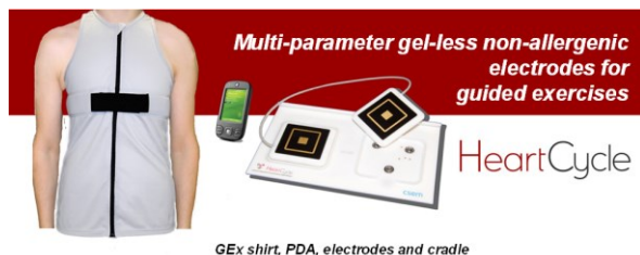
Figure 3: The portable station showing the shirt, the IMAGE sensor and the smart phone (PDA worn on the upper arm) intended for patient guidance during exercising
