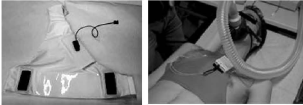
Figure 3. Mini-vest used for thoracic oximetry (left hand side), and setup during hypoxia tests (right hand side)
