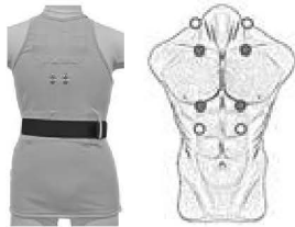
Figure 4. ICG shirt and electrode position
