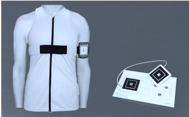
Figure 2. HeartCycle smart ECG electrodes, shirt and smartphone used for guided exercise.
